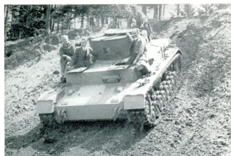
Before turrets were installed, the vehicles were broken in on the factory grounds. A weight was carried equivalent to the weight of the turret. The "Kugelblende 50" ball mount has not yet been installed.
