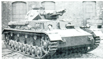
Panzerkampfwagen IV Ausf. D and E were regularly equipped with extra armor plate bolted onto the front and both sides of the superstructure. These photographs show such a vehicle at the Krupp-Grusonwerk in Magdeburg.
