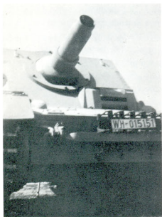
The first series of "Sturmpanzer" were made mounting superstructures on repaired tank chassis that had been returned for major overhaul. These photographs show one of the first series still using the "Fahrrersehklappe 80" of the Tiger I tank. The red registration plates were only used during testing. As a rule, armored full-track vehicles of the German Wehrmacht carried no license plates.
