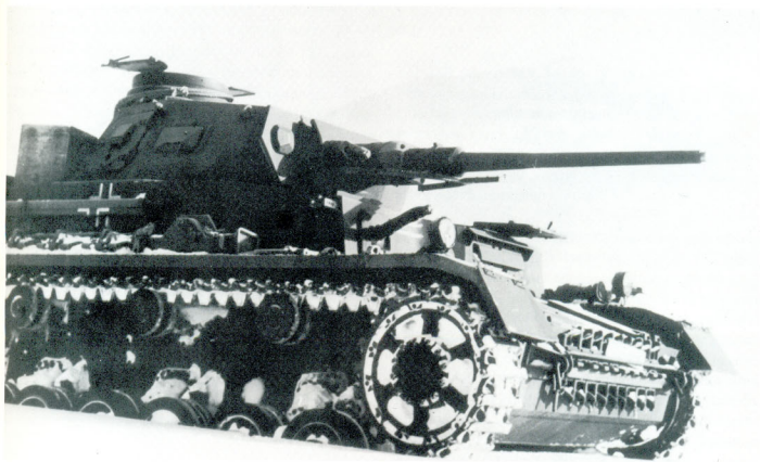
A Panzer IV with the 5 cm KwK 39 L/60 installed as an experiment. This photograph shows the vehicle during winter testing at St. Johann in Tirol, January 13, 1942.
