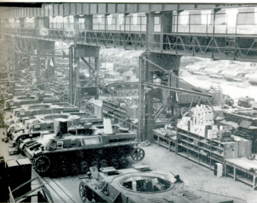
BW tanks on the assembly line in St. Valentin, Lower Austria. The ammunition racks can be seen on the tank in front.
