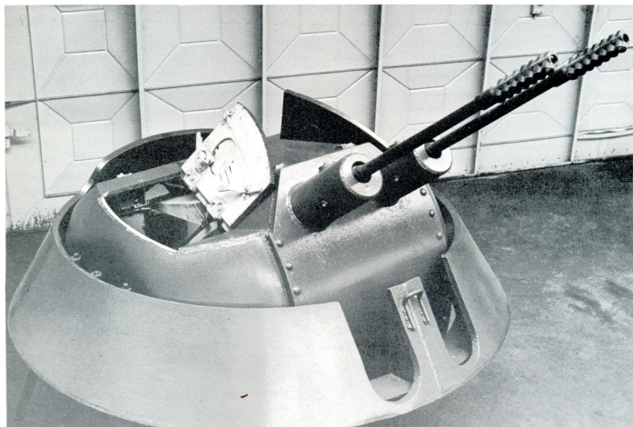
The last turret of the "Kugelblitz" shows the ball housing under its protective cover and the twin guns.
