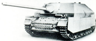
The desire to install the long 7.5 cm 42 L/70 gun in the Jagdpanzer IV resulted in this prototype, which again used an unchanged Panzer IV chassis.
