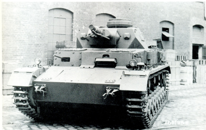
Panzerkampfwagen IV Ausf. D and E were regularly equipped with extra armor plate bolted onto the front and both sides of the superstructure. These photographs show such a vehicle at the Krupp-Grusonwerk in Magdeburg.
