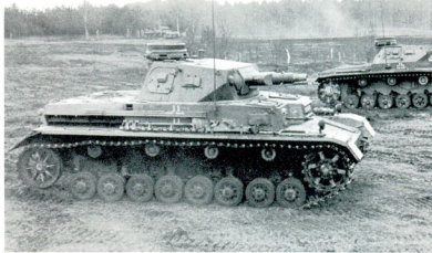
Panzerkampfwagen IV Ausf. D during maneuvers, with a Panzer III in the background. Ausf. D had a stepped superstructure front plate with projecting driver's compartment. The new gun mantle is easy to see.
