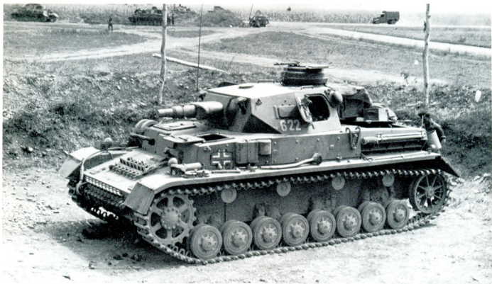
The Panzerkampfwagen IV Ausf. E had new idler wheels and a new design for the commander's cupola. Note also the additional armor plates bolted to the superstructure sides.
