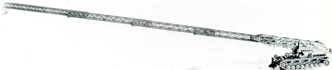
Above: The same model with its bridge extended. The vehicle had to be supported by a hydraulic jack at the front.
