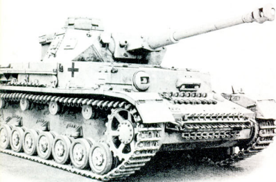
Panzerkampfwagen IV Ausf. G used the 7.5 cm KwK 40 with double chambered muzzle brake. The photographs show three sides of the vehicle.
